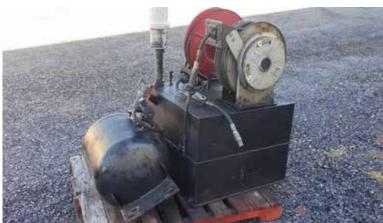
ASPHALT SPRAY UNIT & OIL STORAGE TANK Asphalt Spray Unit,29"x29"x23" & 2 Hose Reels; Waste Oil Tank 200PSI
