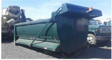
**DUMP TRUCK BODY/BED**17' Steel Tri-Axle Dump Truck Body/Bed with lift cylinder
