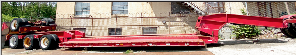
ROGERS SP60DS TRI-AXLE LOWBOY 60-TON HYDRAULIC GOOSE NECK TRAILER
