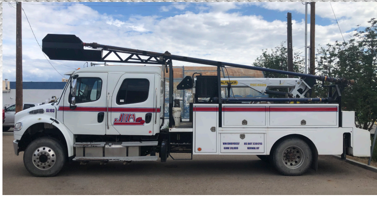
Freightliner | Freightliner Wire line unit, Cummins engine, automatic allison transmission, 23,360 miles, 4427 hrs, Palfinger truck mounted crane with wireless remote. Down hole tools included Plungers, JDC'S, Weight bars, hand tools, air tools, 14,000' slick line. VIN: 1FVDCXBS9DHB0657
