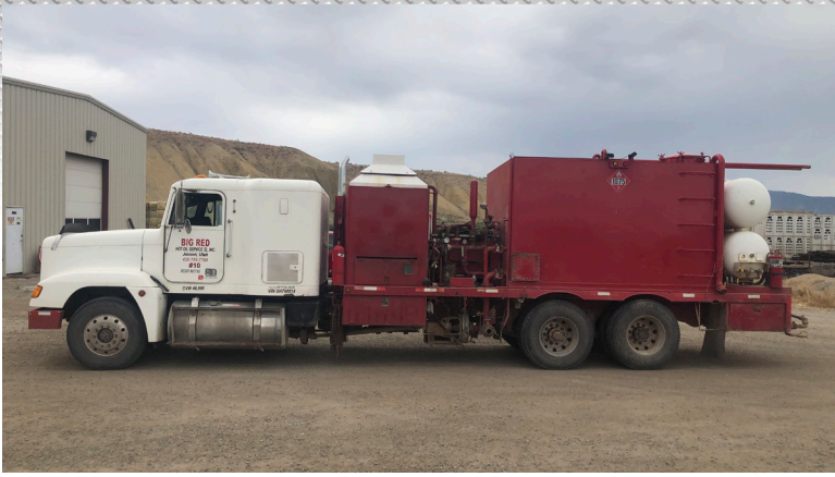
1999 Freightliner | Hot Oil Truck; 7 million Btu, 2x3 centrifugal pump, bowie load pump, gardner denver TEE PE5 5000LB pressure rating with 3 inch plungers, 75 bbl storage tank, high temp automatic shut down and 2 piggy back 250 gallon propane tanks.
