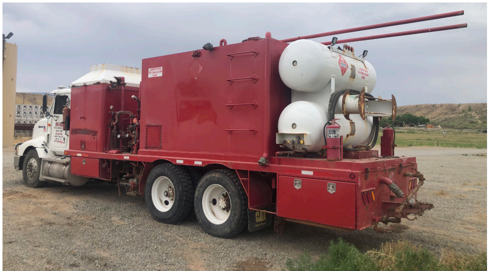
1998 International | Hot Oil truck. Storage Tank, 7 million Btu, 2x3 centrifugal pump, Bowie load pump, Gardner Denver TEE PE5 Pump (5000 lb high pressure rating) with 3" plungers, 75 bbl storage tank, high temp automatic shutdown and 2 piggy back 250 gallon propane tanks.
