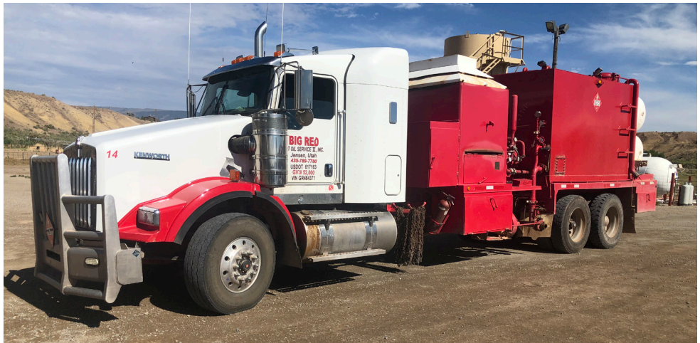
2014 Kenworth | Hot Oil Truck. 7 million BTU'S, 2X3 Centrifugal pump. Bowie load pump, Gardener Denver TEE PE55 pump (5000 lb high pressure rating) with 3" plungers, 75 bbl storage tank with baffles, high temp automatic shutdown and 2 piggy back 250 gallons propane tank. Key way unit
