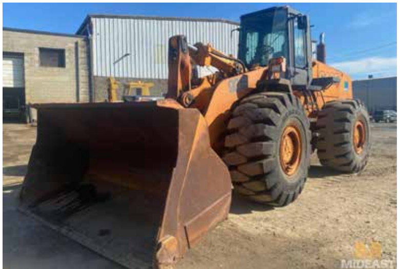
Case 921 B Loader plus Snow Pusher Loader with Snow Pusher, 26.5/25 Tires, E ROPS, 10ft GP Bucket, Cummins eng., s/n JEE0050458
