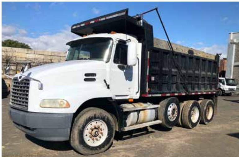
2000 Mack Vision CX613 Tri Axle Dump Truck Miles: 733K, 10 Speed Eaton Fuller, Mack Engine, Tires are fair- 11R 22.5, 17 FT Steel Body, Vin # 1M1AE07Y4YW002120
