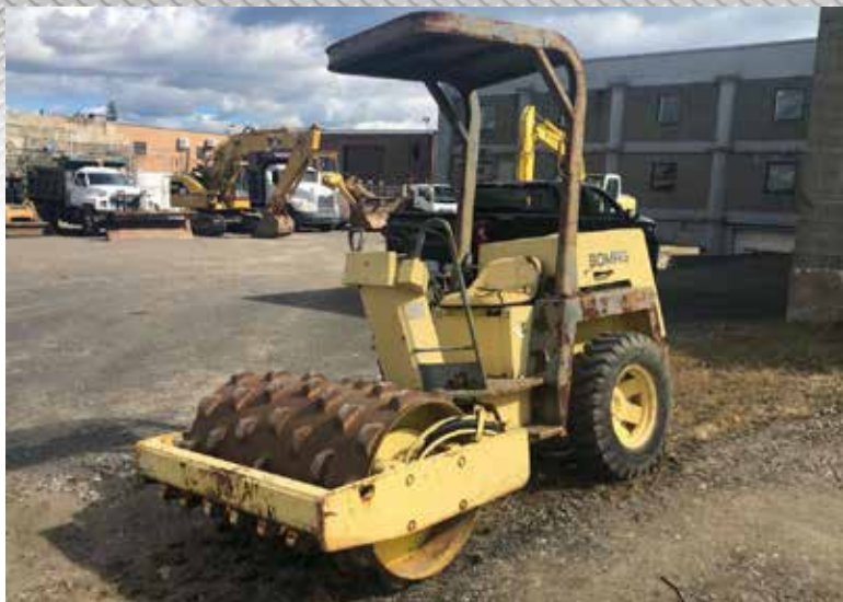
Bomag BW 122PD Vibratory Roller Very Good Condition, Sheeps Foot, s/n 101710100116
