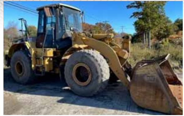
2004 CAT 950G Series II Wheel Loader Hour meter reads 26,663 hrs, A/C, L3 tires, Quick Evac - Engine Prelube, Ride Control, Air Pre-cleaner, with 4 yd bucket. Rebuilt engine 2014 by Milton Cat $ 28,478. s/n AXR00293
