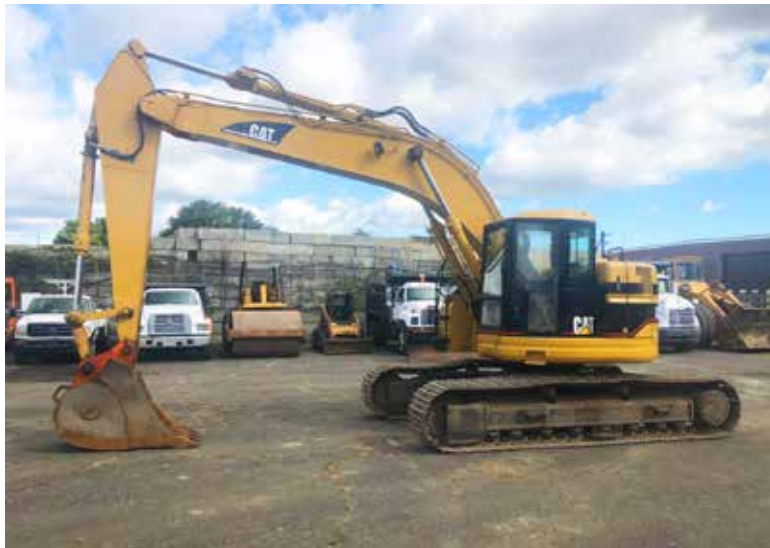
1999 CAT 321C LCR Excavator 9546 hours, 36" Bucket, 24" Pads, s/n 90Z00285
