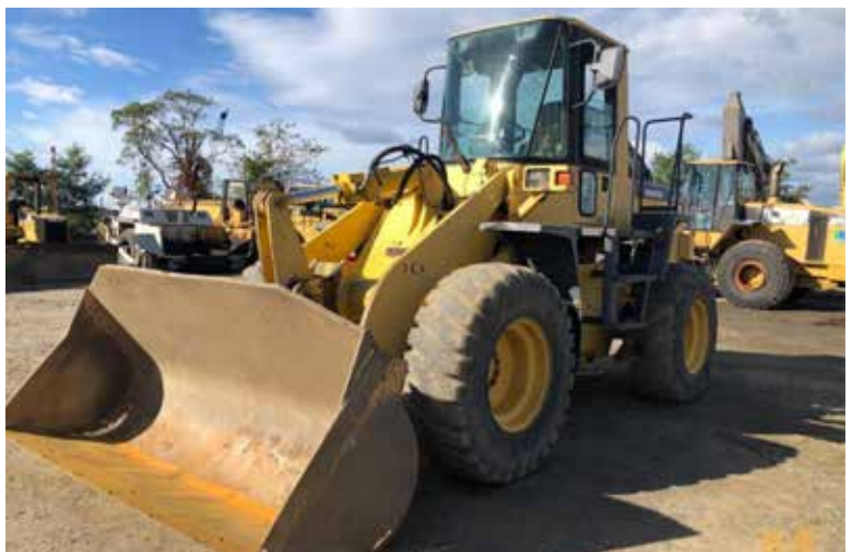
Komatsu WA250-3L Wheel Loader Hours: 112,736, 17.5/25 Tires, E ROPS, 2.5-3.cy, 8.8Ft. GP Bucket, s/n A70525
