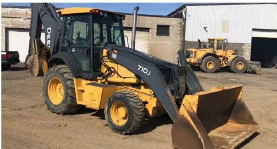
2009 Deere 710J Loader Backhoe | JD710J Super clean, one owner work ready machine. Reading 4,860 Hours. Turbocharged 2240 engine with 4 forward 3 reverse power shift transmission. 26,000 LB operating weight. 8 foot bucket, comes with digging and clean up bucket. Digging depth 17.83 FT. Dig Force 17,000 LB. Reach from swivel 22.5 FT. Load Height 14.25 FT. Tires 14.5/75-16 10PR/15-19.5 8PR. Machine is work ready, needs nothing but work. s/n T0710JX177475
