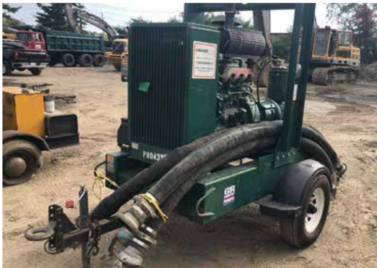
Gorman-Rupp PA4A60-40 Prime Aire Centrifugal Pump s/n 1363296
