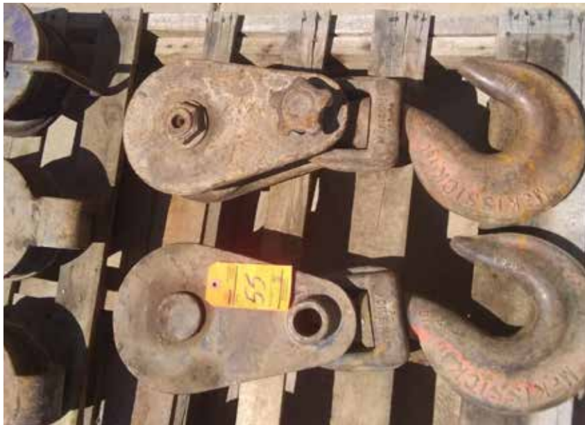
(2) MCKISSICK 20-TON SNATCH BLOCKS WITH SWIVEL HOOKS
