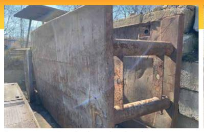
**STEEL TRENCH/SHORING BOXES**1- 14' x 8' x 5', 1-12' x 8' x 8', 1-10' x 6' x 6', 1-8' x 6' x 5'6" w/ lot of pipes
