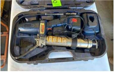
LINCOLN PORTABLE BATTERY-OPERATED GREASE GUN
